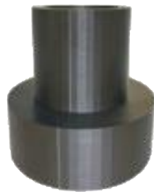
Fig.7- PLA-F 3D printed NSBT using FDM technique
