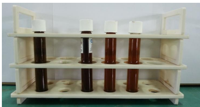
Fig. 8 - The effect of current density on the colour reduction. From left to right: raw leachate, current density of 20, 40 and 60 mA/cm 2 , respectively.
