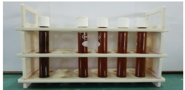
Fig. 4 - The effect of chloride addition on the removal efficiency of colour. From left to right: raw leachate, 2000, 5000, 6000 and 11000 mg/L, respectively.
