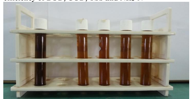
Fig. 2 - The effect of reaction time on the colour. From left to right: Raw leachate, 30, 60, 90, and 120 mins, respectively.
