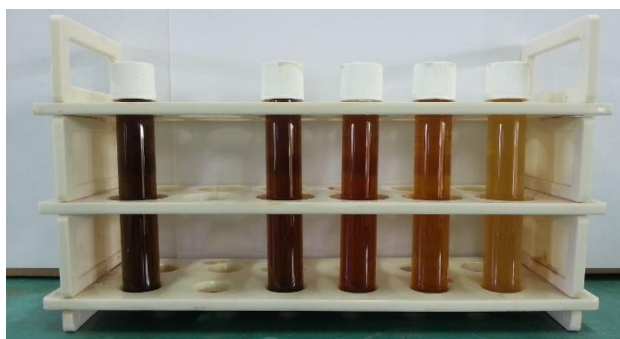
Fig. 6 - The effect of pH on the colour removal. From left to right: raw leachate, pH 8, 7, 6 and 5, respectively.
