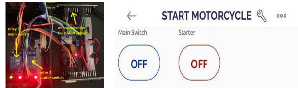
Fig. 6 - Displays Start Motorcycles in Blynk Apps and prototype Start-Stop Engine system
