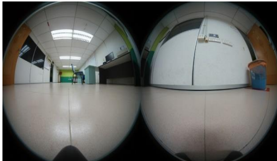
Fig. 4 - Gear 360 dual-fisheye output image (7776 x 3888 pixels). Left half: image taken by the front lens. Right half: image taken by the rear lens
