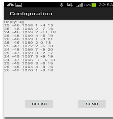
Fig. 7 - Android application for receiving sensor data (accelerometer and gyroscope) from fall detector
